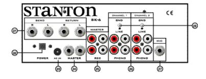
back from the line output of the outboard unit. This creates the effects loop.
